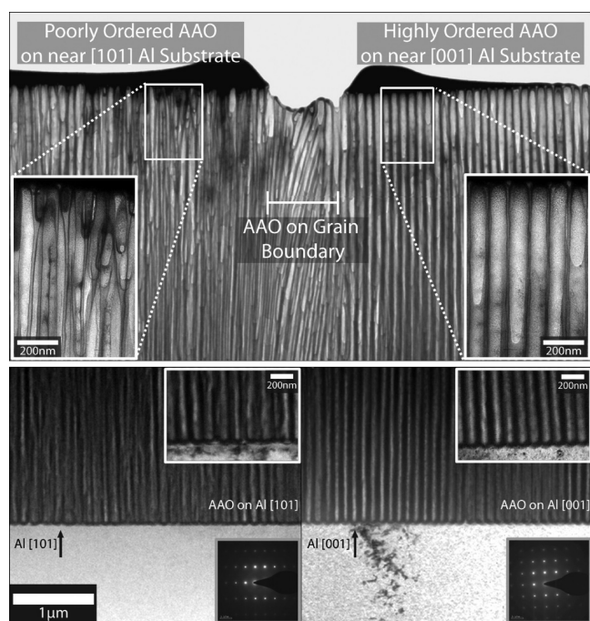
Figure 3. Cross-sectional TEM micrographs showing the longitudinal morphology of the AAO: (a) Cross section near the top surface of the AAO film. (b) Cross section at the metal–oxide junction. The structure shown is grown on top of a grain-boundary region in the Al substrate. The two Al grains on either side of the grain boundary had [001] and [101] orientation, respectively.
